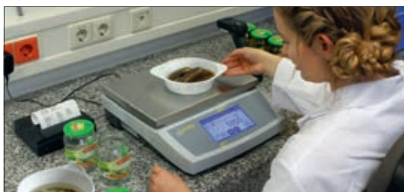
Sample testing of a pre-packaged item which is empty (destructive analysis)
